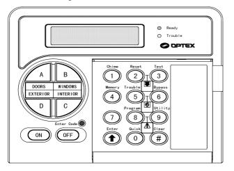
Quad Keys activate pre-assigned zone groups or pre-configured arming modes. Turn on the security system by selecting the appropriate button and pressing 'On'.
