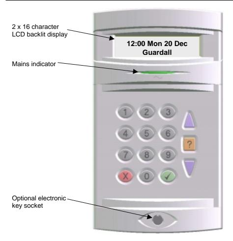
The operator keypad unit incorporates a backlit liquid crystal display (LCD) comprising 2 lines of 16 characters, and a backlit keypad to gain access to the system and to perform all authorised user functions. Keypads may be fitted with an electronic key socket or an internal proximity reader. The keypad incorporates a mains power indicator. This indicator will flash if the system is operating on standby battery power.
