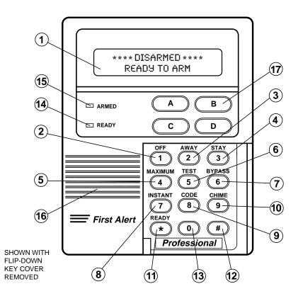
**IMPORTANT!:** When using the keypad to enter codes and commands, sequential key depressions must be made within 3 seconds of one another. If 3 seconds elapses without a key depression, the entry is aborted and must be repeated from its beginning.
