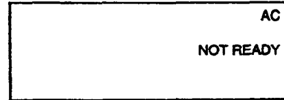
TYPICAL DISPLAY INDICATING OPEN PROTECTION ZONE
