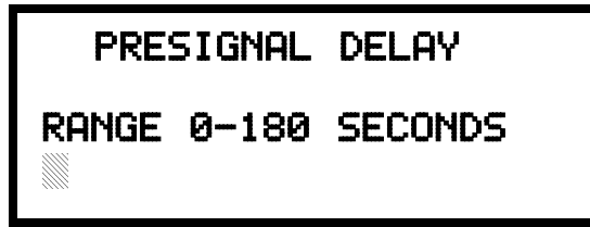
Pre-signal Delay Screen
