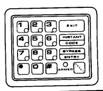
The Keypad REPORTS THE STATUS of your system (armed/disarmed, zone(s) bypassed, trouble) at all times, by means of various lights. You CONTROL THE SYSTEM by gently pressing the appropriate keys.
